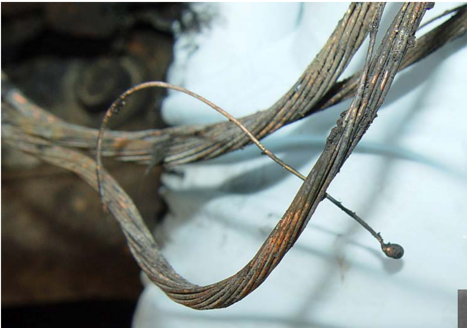
<-Beading seen on copper wire, from auto fire
